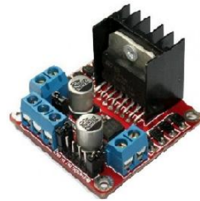
C) Driver Motor Ponte H L298N
